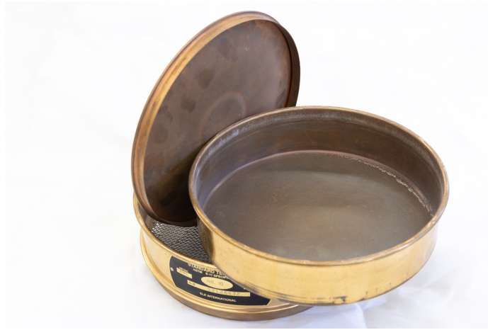
Fig. 5. Examples of the lid (left) and pan (right) that are required for each sieve stack.
