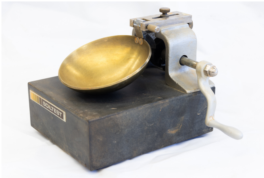
Fig. 17. Example of a manually operated Casagrande cup. The crank is rotated counter-clockwise to lift and drop the brass bowl to impart a small but repeatable impact force into the specimen.
