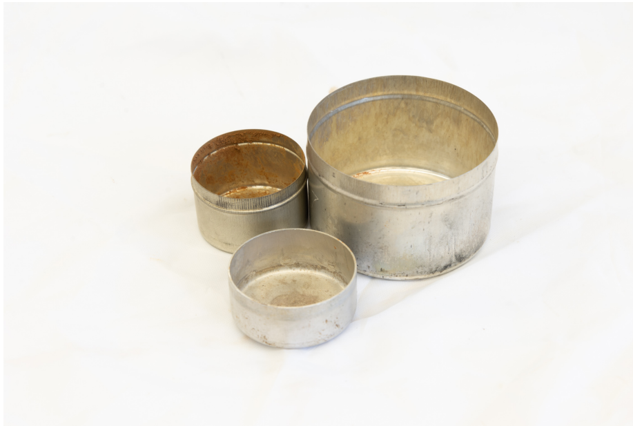
Fig. 16. Aluminum sample containers that can be used for Atterberg limit tests. There is no requirement on the required size of the sample can, just that it can sufficiently hold the material to be oven dried.
