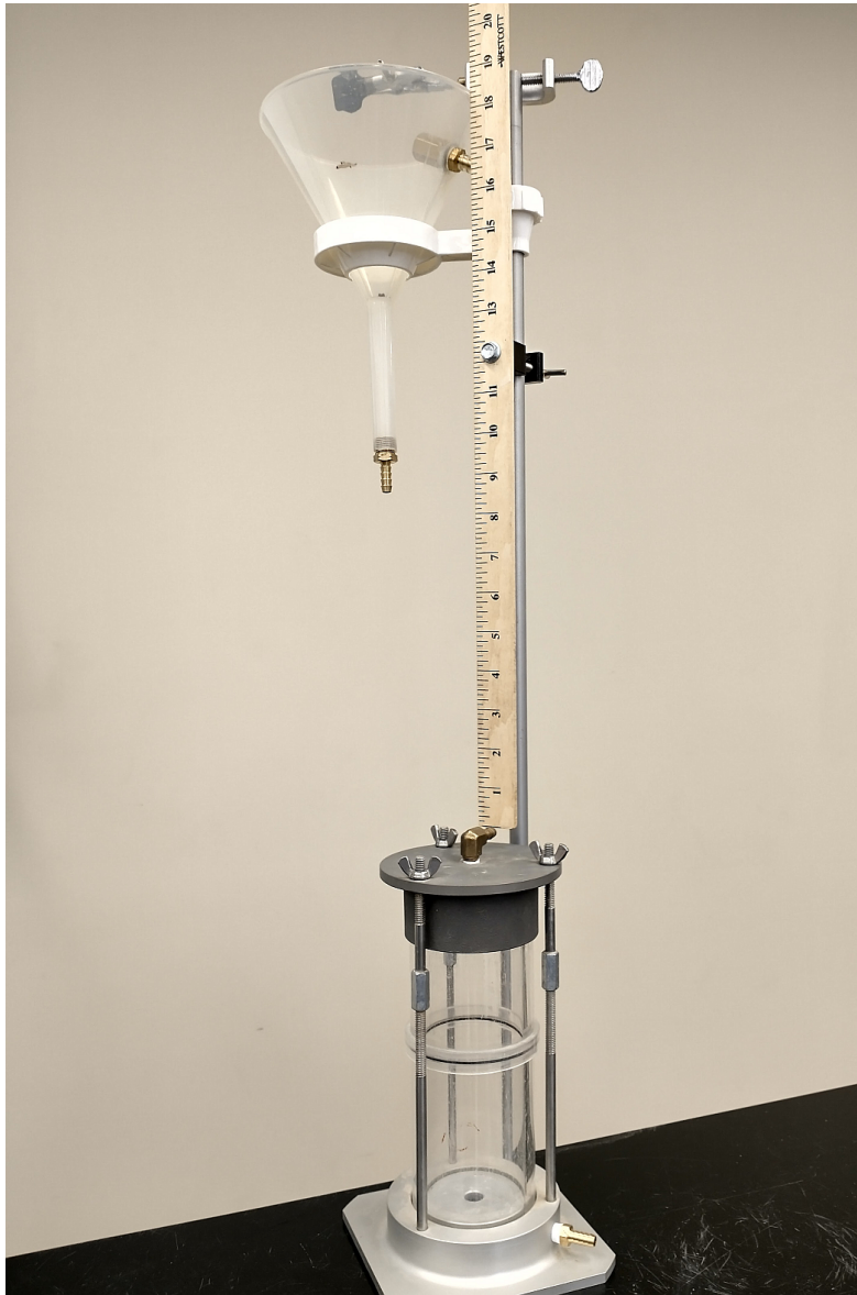
Fig. 25. Permeameter setup used in lab. Note the water tubing is omitted for clarity.
