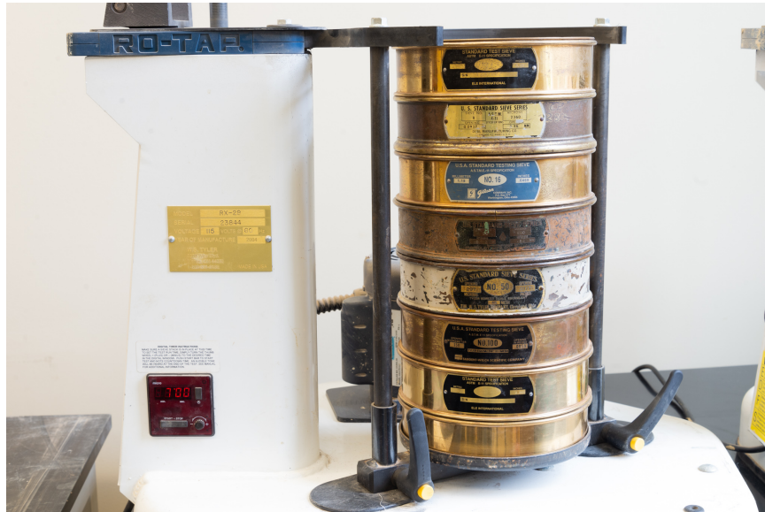
Fig. 9. An example of a sieve stack loaded into a mechanical shaking device and the timer set for 7 minutes.
