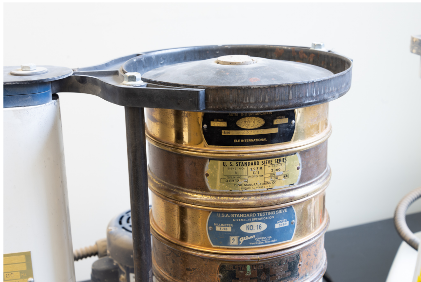
Fig. 10. An example of a sieve stack loaded into a mechanical shaking device and the protective tamping plate placed on top of the sieve stack. The cork or rubber in the center of the plate should be intact. If missing, notify the instructor as damage may occur if not present.
