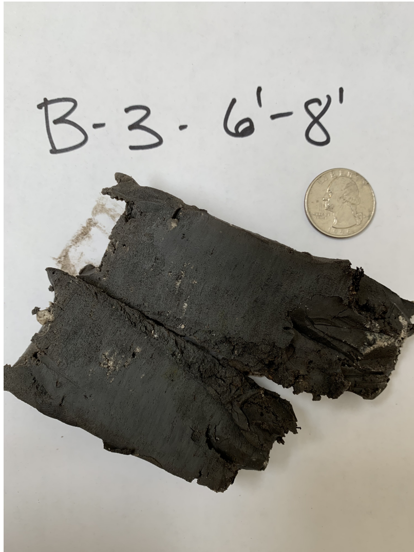
Fig. 1. Example of a predominantly fine-grained (silty lean clay) soil sample. Note how the majority of the particles are too small to see individually. The quarter also offers a quick scale comparison.
