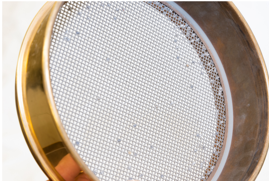
Fig. 6. An example of a #10 sieve with aggregate particles still stuck in the mesh. These should be carefully removed to ensure accurate results.
