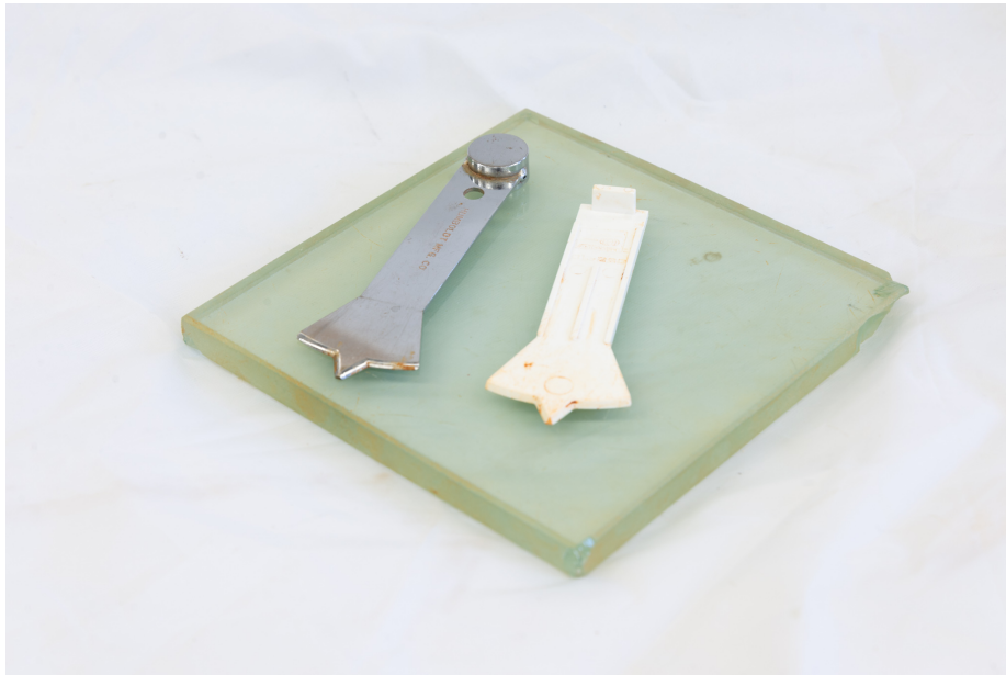
Fig. 18. Example of plastic and metal grooving tools for use in the Casagrande cup. There is a different type of grooving tool that can also be used but will not be utilized for this laboratory exercise.
