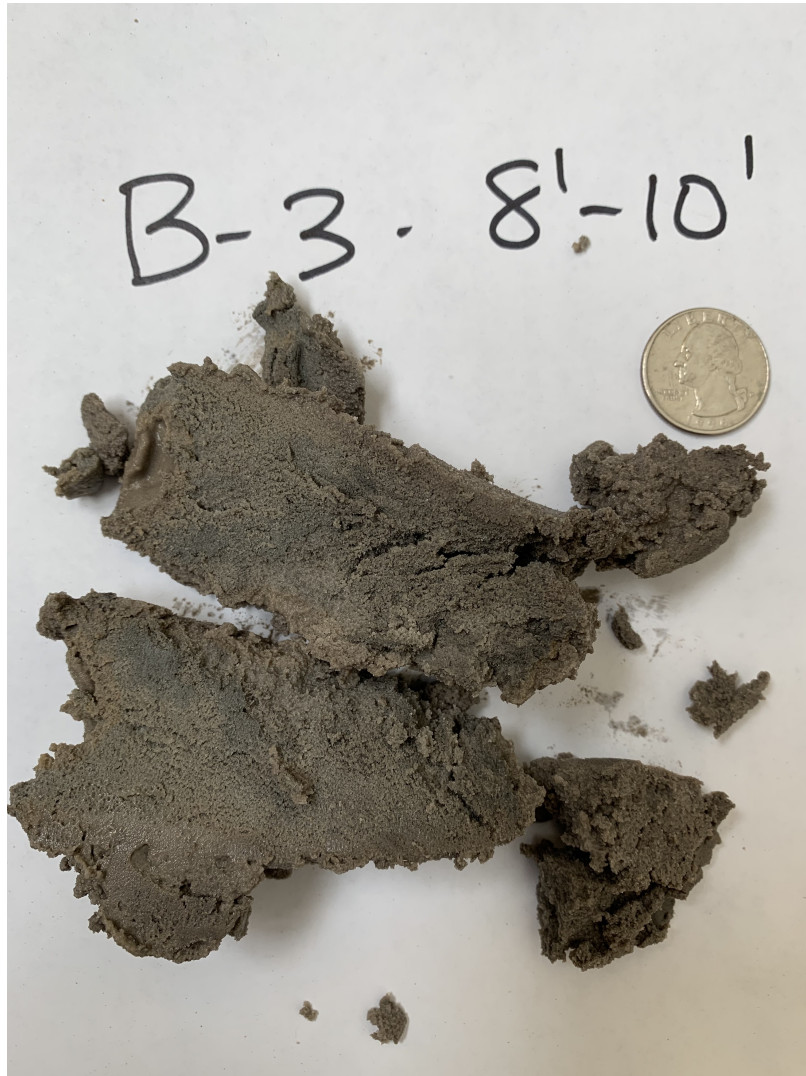
Fig. 2. Example of fine silty sand sample. Note how here we can see many of the individual particles, but they are still quite small. This is a good indication that they are fine sand particles.
