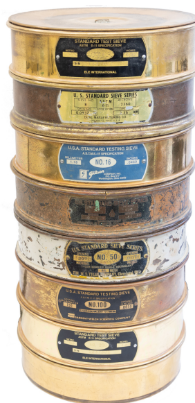
Fig. 8. An example of a properly stacked sieve set. This example is purposely made up of sieves from various companies and ages to demonstrate the variety in the nameplates. Even the ugly ole #30 sieve needs some lovin'.
