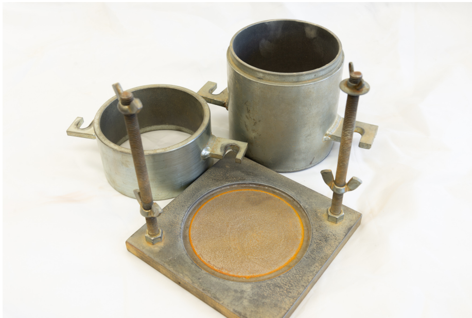
Fig. 21. Example of a 4-inch diameter proctor mold. The taller piece goes on first followed by the shorter piece.
