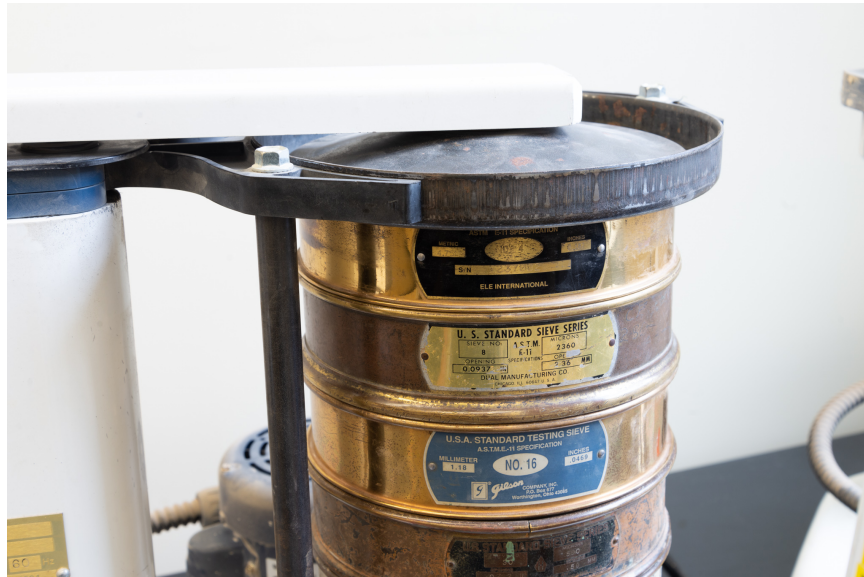
Fig. 11. An example of a sieve stack loaded into a mechanical shaking device and the protective tamping plate placed on top of the sieve stack with the tamping arm from the shaker resting on the tamping plate. At this point, the sieve stack is ready to be mechanically shaken, not stirred.
