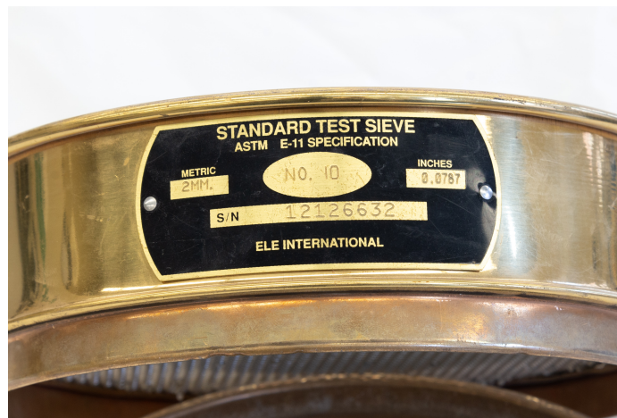
Fig. 4. Example of sieve nameplate. This is a #10 sieve which has an opening of 2 mm or 0.0787 inches. Note that the ASTM E11 designation is also indicated.
