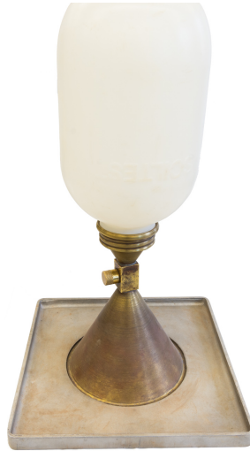
Fig. 23. Assembled sand cone apparatus sitting on a base plate.
